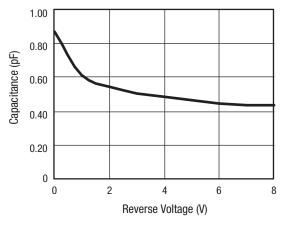
Figure 2. SMS3922 Series Total Capacitance vs Reverse Voltage
