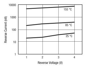
Figure 5. SMS3922 Reverse Current vs Reverse Voltage
