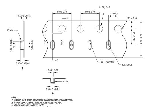
Figure 10. SC-79 Tape and Reel Dimensions
