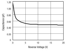
Figure 3. SMS3923 Series Total Capacitance vs Reverse Voltage
