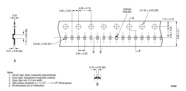
**Figure 18. SOD-882 Tape and Reel Dimensions**
