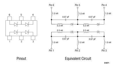
Figure 1. SMS3923-081 Dual Series Pair Pinout and Equivalent Circuit
