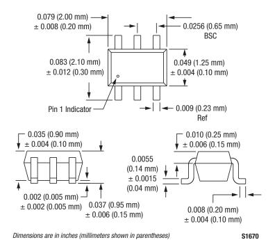
Figure 11. SC-88 Package Dimension Drawing
