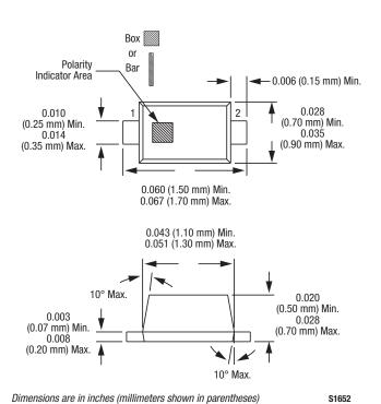
Figure 9. SC-79 Package Dimension Drawing
