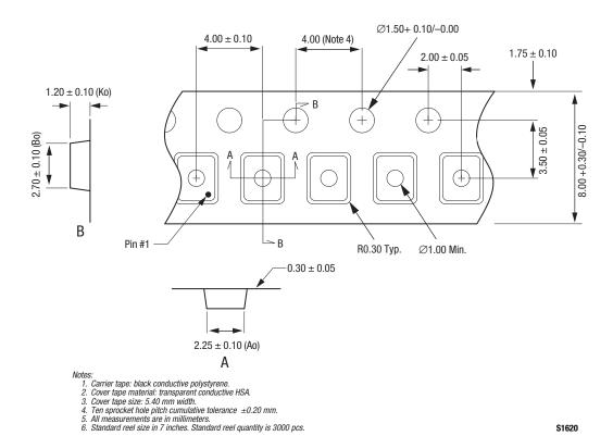
Figure 12. SC-88 Tape and Reel Dimensions
