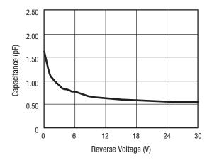
Figure 4. SMS3924 Total Capacitance vs Reverse Voltage
