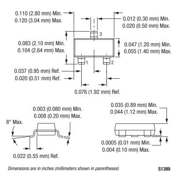
Figure 13. SOT-23 Package Dimension Drawing
