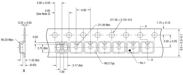
s: Carrier tape: black conductive polycarbonate. Cover tape material: transparent conductive PSA. Cover tape size: 5.4 mm width. Tolerance: XX = ±0.10 Ten sprocket hole pitch cumulative tolerance: ±0.2 mm. All measurements are in millimeters.
