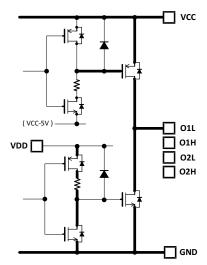
Figure 7. O1L, O1H, O2L and O2H Equivalent Circuit
