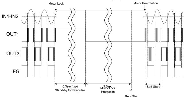
Re - Start Figure 33. Image of Lock Detection and Lock Protection
