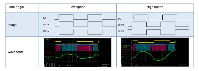
Figure 29. Lead Angel Image Waveform
