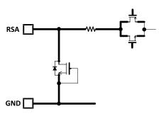
Figure 15. RSA, RSB Equivalent Circuit
