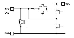
Figure 12. SFS, LAG Equivalent Circuit
