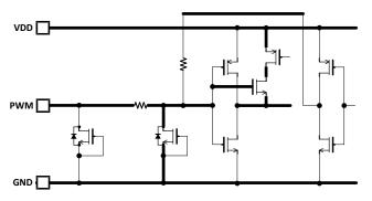
Figure 17. PWM Equivalent Circuit
