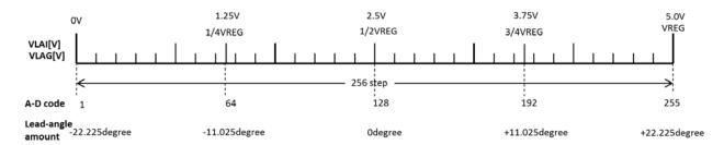
Figure 27. Lead-Angle Parameter Setting for LAI/LAG Pin
