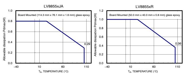
Figure 5. Power Dissipation vs Ambient Temperature Characteristic
