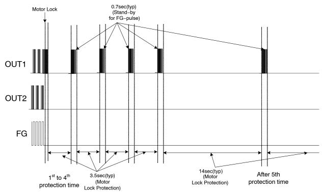
Figure 34. Image of Lock Protection Time
