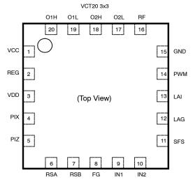
Figure 4. LV88551R, LV88552R, LV88553R, LV88554R Pin Assignment
