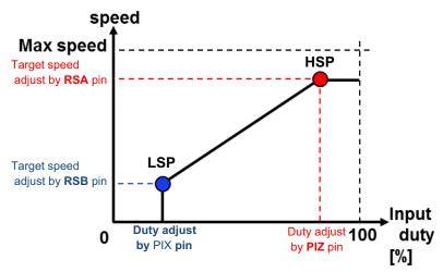
Figure 22. Speed Setting Curve Type Example 2
