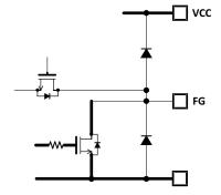
Figure 16. FG Equivalent Circuit
