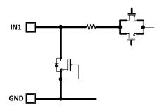
Figure 11. IN1, IN2 Equivalent Circuit
