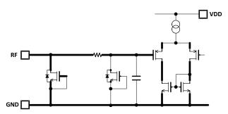
Figure 18. RF Equivalent Circuit
