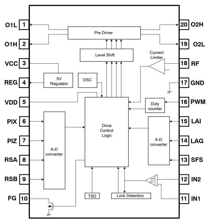
Figure 1. LV88551JA, LV88552JA, LV88553JA, LV88554JA Block Diagram
