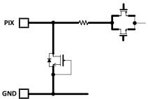
Figure 14. PIX, PIZ Equivalent Circuit
