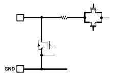
Figure 13. LAI Equivalent Circuit
