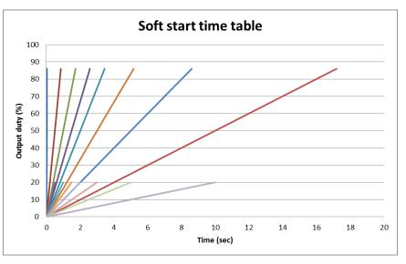
Figure 30. Soft-start and Dead Time Setting Table for SFS Pin
