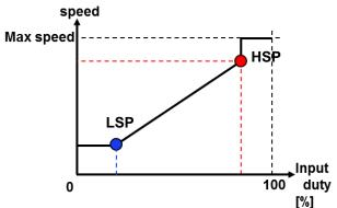
Figure 20. Image of Speed Setting Curve
