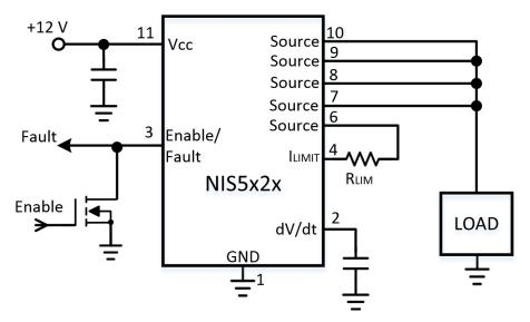
Figure 2. Application Circuit with Kelvin Current Sensing
