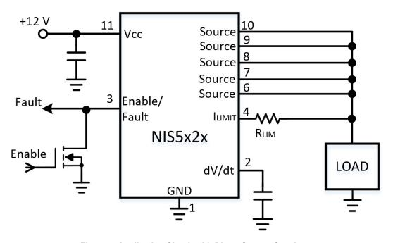
Figure 4. Application Circuit with Direct Current Sensing
