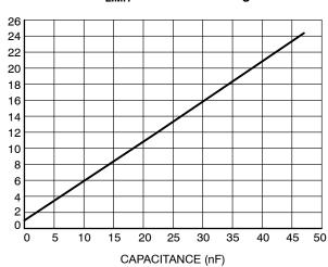
Figure 9. Output Voltage Ramp Time vs. dv/dt Capacitance
