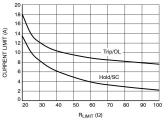
Figure 7. NIS5020/NIS5021 Current Limit vs. R<sub>LIMIT</sub> for Kelvin Sensing
