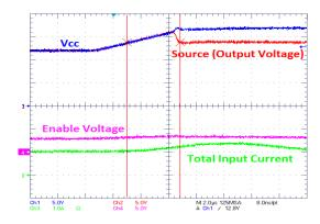
Figure 11. NIS5020 Overvoltage Clamp Operation
