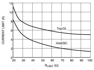
Figure 8. NIS5820 Current Limit vs. R<sub>LIMIT</sub> for Kelvin Sensing
