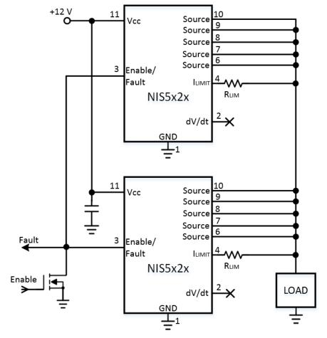
Figure 5. Paralleling eFuses
