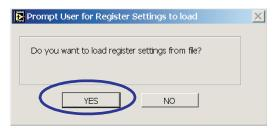
Clicking on the *YES* button prompts the user to select the register setting file from an existing directory (as shown below) that has previously been used to save the files. From this window, the user can navigate, and select the correct file to write to the device. Confirm the file selected by clicking on the *OK* button. Once the file to be written to the device is selected, the Write to Configuration Register button must be pressed to complete the write command to the AMC6821 device.
