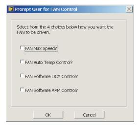
The step-by-step dialog as shown in the series of splash screens above is provided to guide the user, and ensure that the correct setup or configuration, based on the fan that is used, is achieved. All other registers that are not touched by the bit settings, as a result of the selections made from the series of splash screens, assume the default values.
