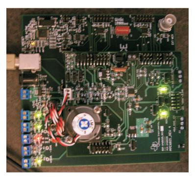
Figure 11. AMC6821EVM and USB-MODEVM Hardware Setup
