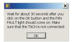
Click on the *OK* button and the progress bar should start to show activity. When the progress bar reaches its full range as shown below, the FAN-FAULT alarm should turn red. At this point all alarms should be turned red. The FAN-FAULT alarm LED indicator, D3, on the EVM should turn on as well, but it may turn on earlier than the software indicator.
