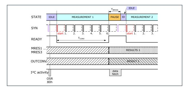
The conversion time ( $T_{CONV}$ ) is determined by the duration between the edges of the start and stop of the SYN signal. If CREG2:EN\_TM is set to "1", the register OUTCONV contains an equivalent amount of  $T_{CONV}$  as counts of the internal clock. With the value of OUTCONV, the measurement results can be calculated more precisely (see chapter 7.6).
