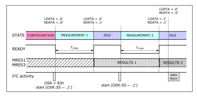
The status bits, STATUS:STANDBYSTATE and STATUS:POWERSTATE, always show the actual status of the internal control signals for Standby and Power Down. In both cases, it can differ from the actual set bits CREG3:SB and OSR:PD, due to the behavior of the control signals while a measurement is in process. The reading of the 16-bit values of the output result registers always starts with the least significant byte.
