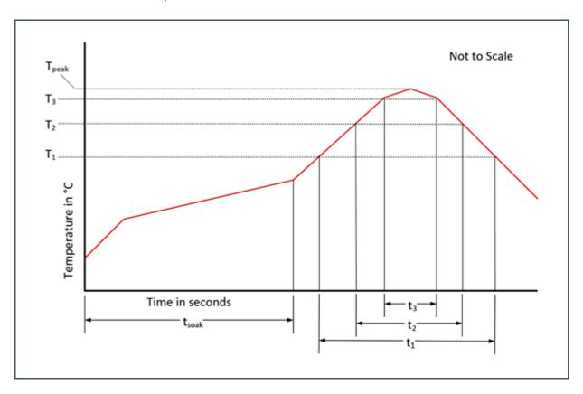
Figure 63: Solder Reflow Profile
