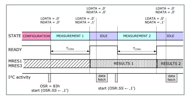
If the buffer registers contain new values (NDATA = "1") and new measurement finishes before an I<sup>2</sup>C reading process occurs, the new measurement results are stored in the buffer registers. The older measurement results are overwritten. The status bit, LDATA, shown in Figure 57 indicates this. The LDATA bit is only reset to "0" by reading the status register, as it allows checking for the loss of information after multiple measurement cycles.
