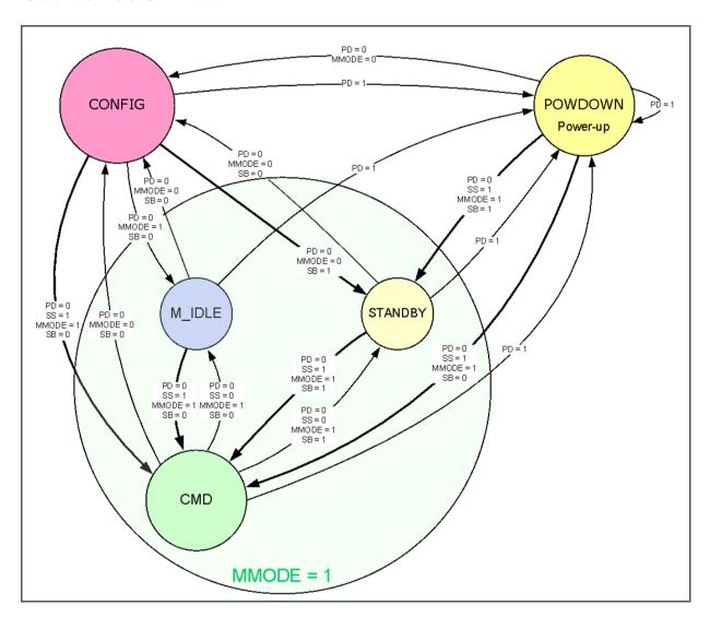
Figure 15 shows the principle sequence for a measurement to start in CMD mode coming from the Configuration state and waiting in the Measurement state between the measurements is shown as IDLE:
