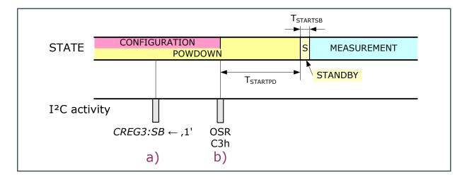
Figure 19 shows the principle start of the measurement from OSR:PD = "1" and CREG3:SB = "1":
