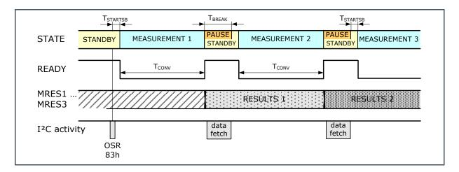
Another example shows, that after the end of a conversion in CMD mode the AS7331 returns to power down and/or standby state depending on the bits OSR:PD and CREG3:SB. In case of both bits are "0" while the measurement state the device would return to idle, waiting for the next measurement to start. Figure 22 shows the principle sequence whereas measurement starts in CMD mode with power down and standby switched on (device is already in measurement state):
