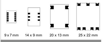
Industry's smallest 9.0 x 7.0 x 6.5H mm OCXO, plus 3 industry standard packages for drop-in replacement of quartz
