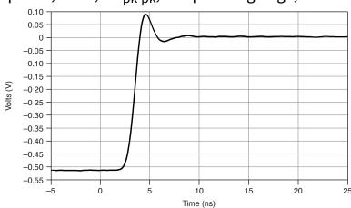
Figure 4. Step Response, 1 M $\Omega$ , 1 V $_{pk-pk}$ , 500 ps Rising Edge, Measured
