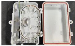
9. Feed the fibers around the outer oval of the splice tray.
