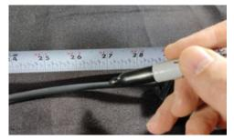
4. Measure 27-inches from the end of the cable an make a mark with a black marker. Feed the grommet over the cable beyond the mark on the cable jacket.
