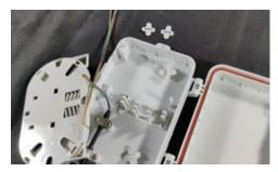
10. Flip the splice tray over and remove the cable "T" under the hinged area of the splice tray and the top of the distribution box.
