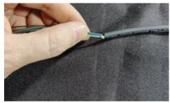
5. Remove the jacket at the mark and cut off the aramid fiber.
