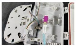
12. Remove the patch cable grommet from the bottom of the distribution box. Insert a fiber optic coupler into the base of the distribution box and connect the patch cable into the coupler.
