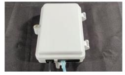
18. Close the distribution box making sure there is an audible click from the side clips. Secure the box with the security hex bolt. Mound the box onto the wall.
