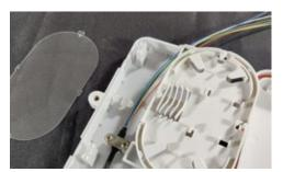
8. Using a flathead screwdriver, carefully pry upward between the hinge of the splice tray to remove it from the distribution box. Remove the clear cover of the splice tray.
