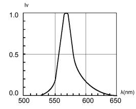
Fig. 1 Relative Luminous Intensity vs. Wavelength
