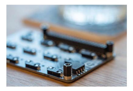
You can now push your Keybow PCB's female GPIO header down onto the male GPIO pins on the Zero WH. Make sure that all the pins are lined up correctly. There will be a little gap left between the headers, but don't worry because they'll still be making good electrical contact.
