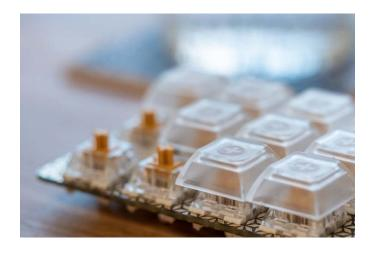
Flip the switch plate with switches and key caps mounted and take a look at all of the pins on the switches. Sometimes, they can get bent slightly in transit, but they all need to be straight to fit correctly into the hot-swap sockets. You can gently bend them back into position if you need to.
