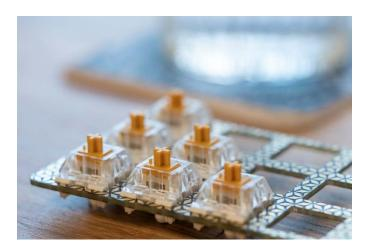
Next, we'll mount the key caps. It doesn't matter which way round they go, as they're completely symmetrical. Push them all the way down onto the stems on the switches.
