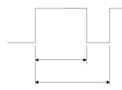
HIGH SIGNAL:5.0 VDC MAX.<br/>2.8 VDC MIN.LOW SIGNAL:0.5 VDC MAX.<br/>0.0 VDC MIN.DUTY CYCLE= $\frac{t}{T}$  \*100(%)
