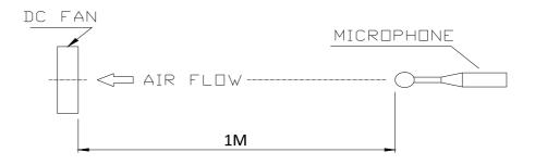
NOISE IS MEASURED AT RATED VOLTAGE IN FREE AIR IN ANECHOIC CHAMBER WITH B & K SOUND LEVEL METER WITH MICROPHONE AT A DISTANCE OF ONE METER FROM THE FAN INTAKE.
