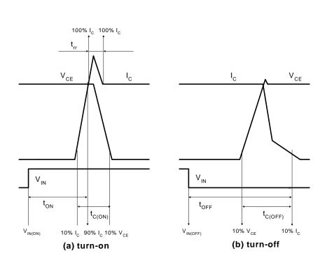
Figure 4. Switching Time Definition
