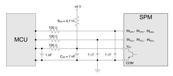
Figure 11. Recommended MCU I/O Interface Circuit
