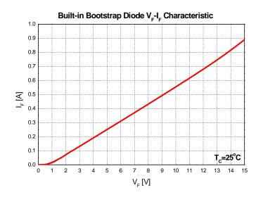
Figure 6. Built-in Bootstrap Diode Characteristics
