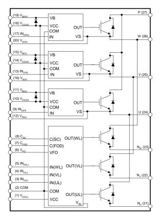
Figure 3. Internal Block Diagram
