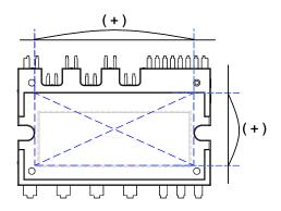
Figure 7. Flatness Measurement Position
