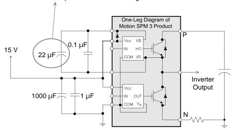
Figure 12. Recommended Bootstrap Operation Circuit and Parameters
