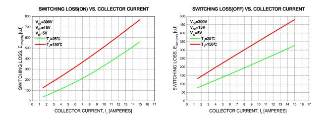
Figure 5. Switching Loss Characteristics (Typical)
