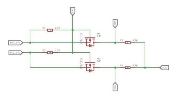
This is a typical Bi-directional level shifter circuit to connect two different voltage section of an I<sup>2</sup>C bus. The I<sup>2</sup>C bus of this sensor use 3.3V, if the I<sup>2</sup>C bus of the Arduino use 5V, this circuit will be needed. In the schematic above, **Q6** and **Q5** are N-Channel MOSFET 2N7002A, which act as a bidirectional switch. In order to better understand this part, you can refer to the AN10441
