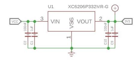
The typical voltage of AMG8833 is 3.3V, so we use the XC6206P33 chip to provide a stable 3.3V. The input of XC6206P33 ranges from 1.8V to 6.0V, so you can use this module with your Arduino both in 3.3V and 5V.
