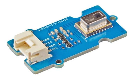
The Grove - Infrared Temperature Sensor Array (AMG8833) is a high precision infrared array sensor which based on advanced MEMS technology. It can support temperature detection of two-dimensional area:  $8 \times 8$  (64 pixels) and maximum 7 meters detection distance.
