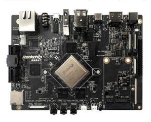
Support TensorFlow / Caffe / Mxnet Support 8bit/16bit operation Up to 3.0TOPs
