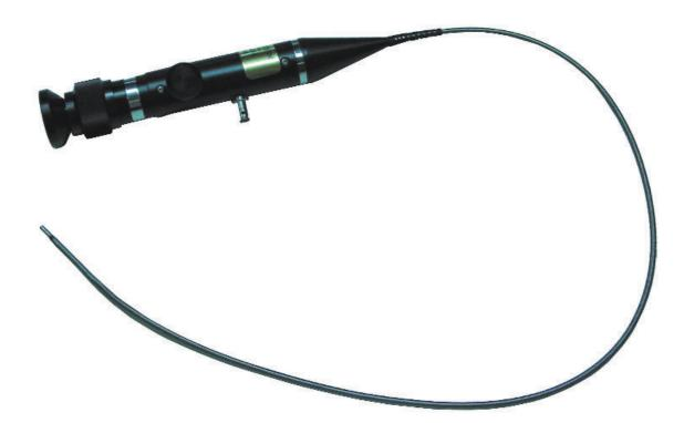
J Series flexible borescopes are two-way articulating borescopes featuring a small diameter of only 0.120" (3.0mm). It offers the high resolution of 10,000 fibres with 25X magnification and is adaptable to video viewing or digital photography. Fibreoptic illumination and a 90° right-angle viewing head are optionally available.
