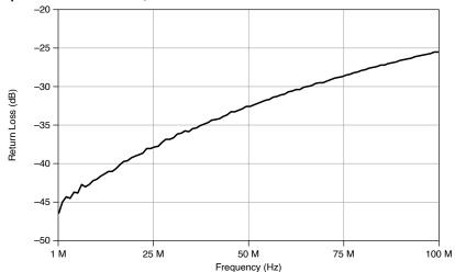
Figure 2.  $50\,\Omega$  Input Return Loss, Measured
