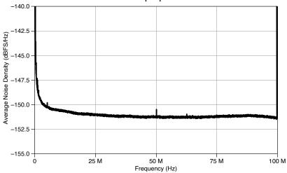
Figure 6. 50  $\Omega$  Average Noise Density, 0.2  $V_{pk\text{-}pk}$  Range, Measured
