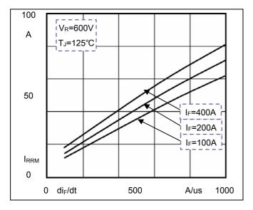
Fig3. Reverse Recovery Current vs di<sub>F</sub>/dt
