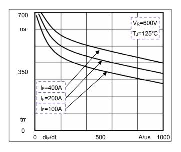
Fig2. Reverse Recovery Time vs di<sub>F</sub>/dt
