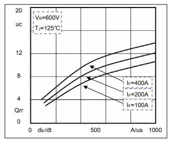
Fig4. Reverse Recovery Charge vs di<sub>F</sub>/dt
