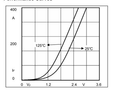
Fig1. Forward Voltage Drop vs Forward Current
