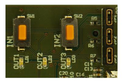
Figure 4. LEDs and buttons
