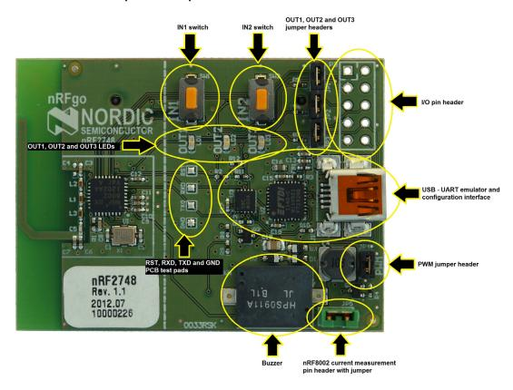
Figure 2. nRF2748 top view
