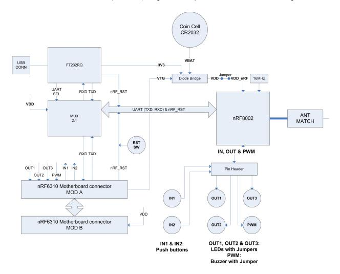
Figure 9. nRF8002 Block diagram
