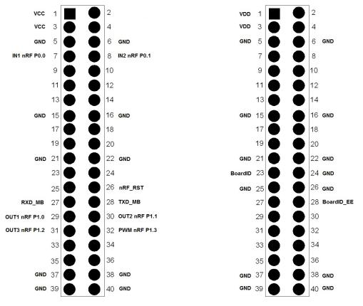
Figure 7. Pinouts for the nRF2748 module connector, P1 (Left) and P2 (Right)
