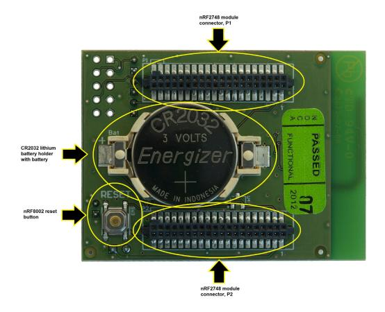
Figure 3. nRF2748 bottom view
