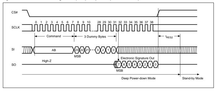
Figure 24. Release from Deep Power-down (RDP) Sequence (Command AB)
