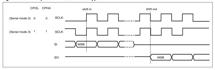
Figure 1. Serial Peripheral Interface Modes Supported
