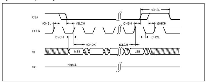
Figure 8. Output Timing
