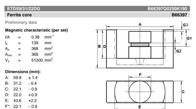
\* These dimensions will be passed through a sorting gauge as a measure of alignment between the glued parts.
