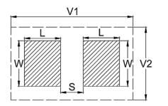
**Density Level A:** For low-density product applications. Recommended for wave solder applications and provides a wider process window for reflow solder processes. **Density Level B:** For products with a moderate level of component density. Provides Recommended Profile Conditions for reflow solder processes.
