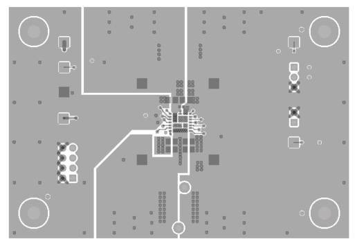
Figure 3 Board layout - layer 1
