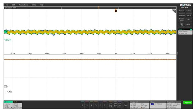
Figure 14  $V_0$  ripple at 12A (Ch1: $I_0$ , Ch8:  $V_{0UT}$ ), peak-peak  $V_0$  ripple = 4.6mV
