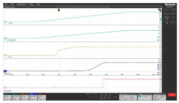
Figure 8 Startup with no load (Ch2:PV<sub>IN</sub>, Ch5:V<sub>CC</sub>, Ch6: V<sub>OUT</sub>, Ch7: PGood, Ch8: Enable)
