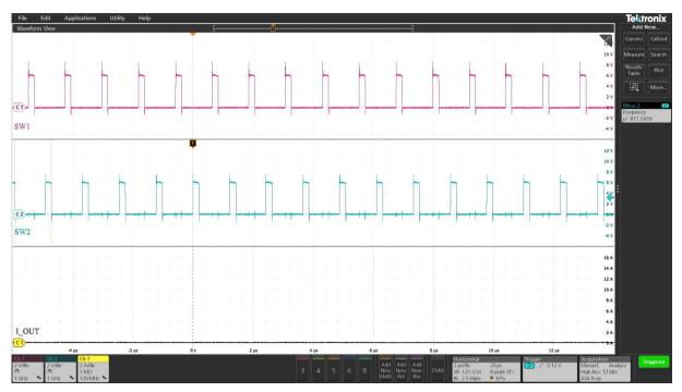
Figure 12 Switch node waveforms at no load
