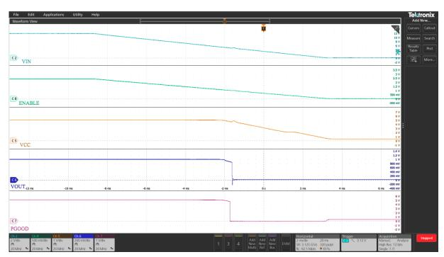
Figure 10 Shutdown with Enable de-assertion at 12A load (Ch2:PV<sub>IN</sub>, Ch5:V<sub>CC</sub>, Ch6: V<sub>OUT</sub>, Ch7: PGood, Ch8: Enable)
