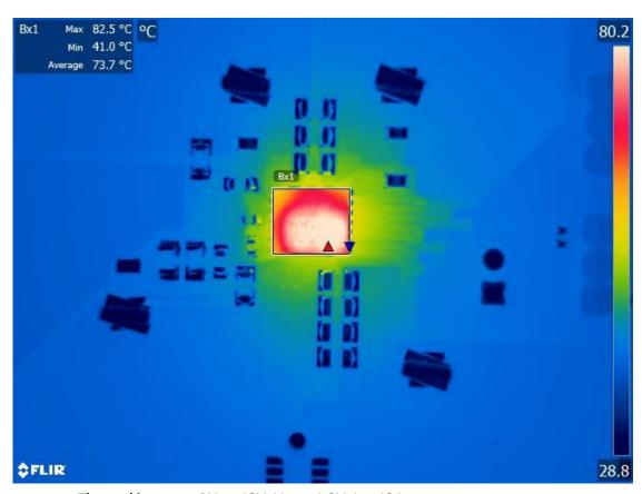
Figure 19 Thermal image at  $PV_{IN} = 12V$ ,  $V_{OUT} = 1.0V$ ,  $I_O = 12A$ , room temperature, no airflow, FS1412 maximum temperature rise = 55.5°C
