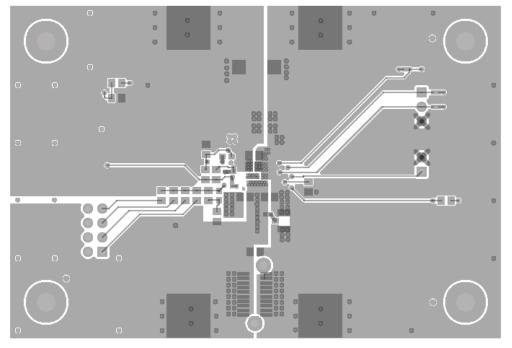
Figure 6 Board layout - layer 4
