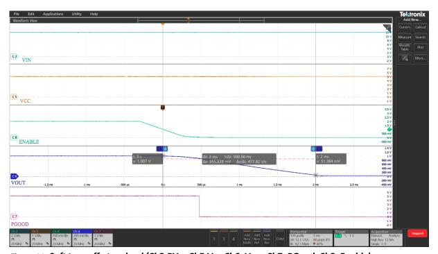
Figure 11 Soft turn off at no load (Ch2:PV<sub>IN</sub>, Ch5:V<sub>CC</sub>, Ch6: V<sub>OUT</sub>, Ch7: PGood, Ch8: Enable)
