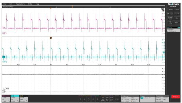
Figure 13 Switch node waveforms at 12A
