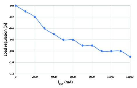
Figure 18 Load regulation ( $I_{0} = 0-12A$ )
