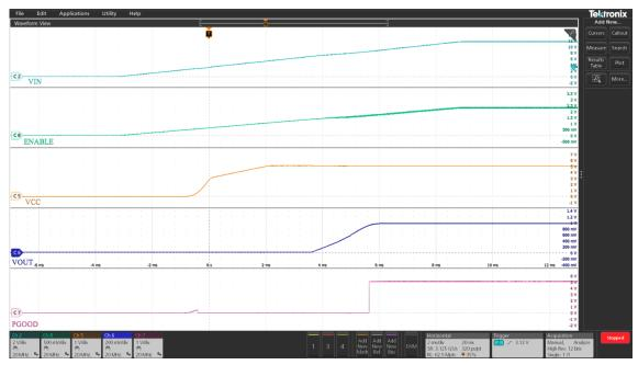
Figure 9 Startup with 12A load (Ch2:PV<sub>IN</sub>, Ch5:V<sub>CC</sub>, Ch6: V<sub>OUT</sub>, Ch7: PGood, Ch8: Enable)
