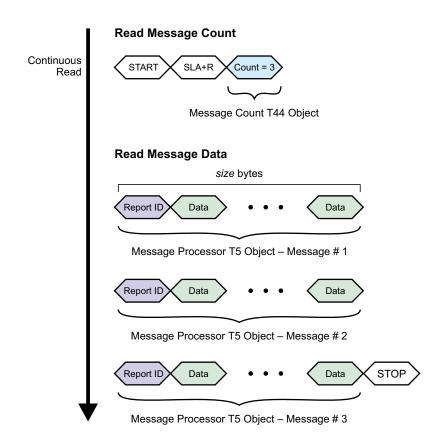
FIGURE 7-10: CONTINUOUS MESSAGE READ EXAMPLE – I<sup>2</sup>C CHECKSUM MODE Set Address Pointer
