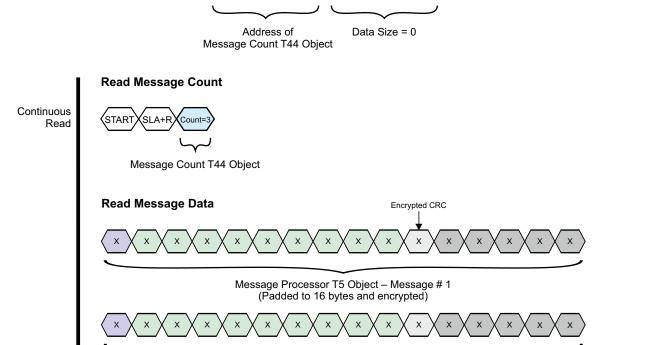
Message Processor T5 Object – Message # 2 (Padded to 16 bytes and encrypted)
