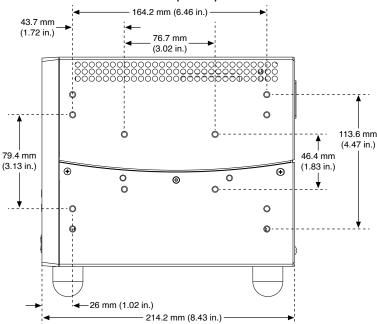
Figure 2. PXIe-1083 Chassis Dimensions (Side)
