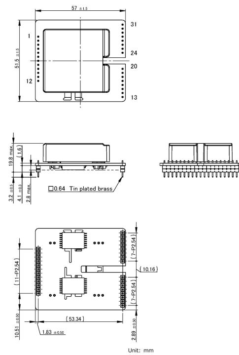
Note: 1. The dimensional tolerance without directions is  $\pm$  0.5mm.
