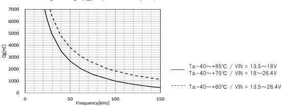
Total gate charge (Qg) vs permissible frequency curve
