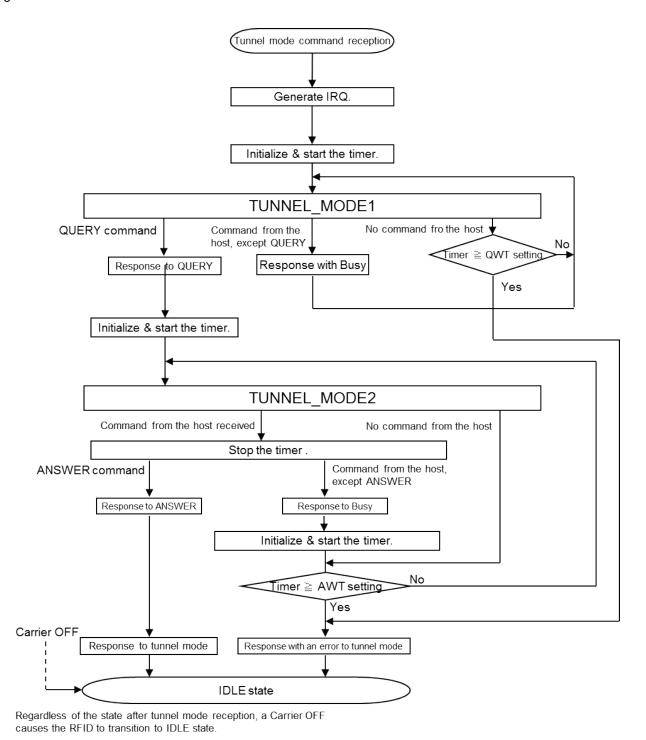
Figure 8-4 Flow Chart in Tunnel Mode
