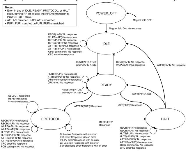
Figure 4-21 State Transtion Diagram for Operation Based on ISO/IEC14443 TypeB
