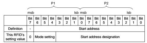
Figure 4-26 Address Specification
