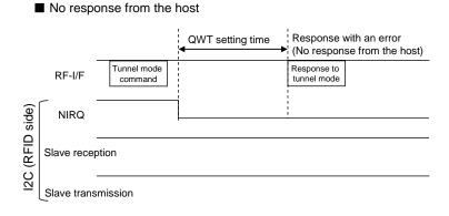
Figure 7-4 Timeout of Waiting for QUERY Command (No Response from the Host)
