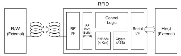
Figure 1-1 Block Diagram
