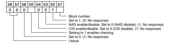
Figure 4-16 I-block Coding
