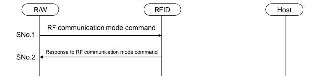
Figure 4-1 RF Communication Mode Sequence
