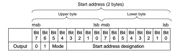
Figure 7-2 Address Setting for Response to QUERY Command
