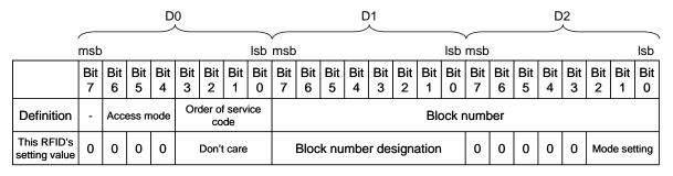
Figure 4-10 Block Element of 3 Bytes
