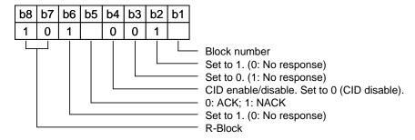
Figure 4-17 R-block Coding
