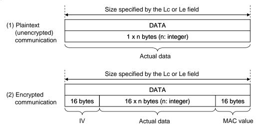
Figure 4-27 Data Block Structure
