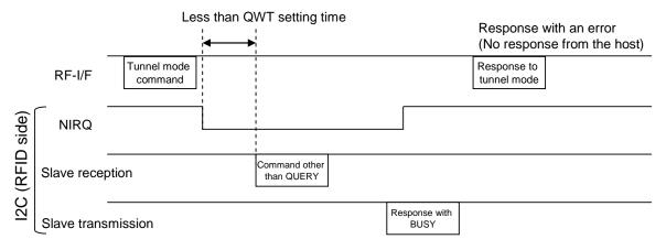
Figure 7-5 Timeout of Waiting for QUERY Command (Command Other Than QUERY)
