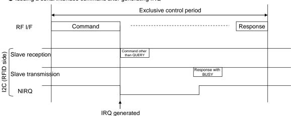
Figure 8-2 Exclusive Control in Tunnel Mode
