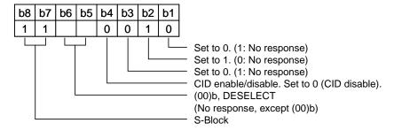
Figure 4-18 S-block Coding
