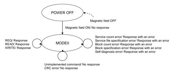
Figure 4-3 State Transition Diagram of JISX6319-4 PICC
