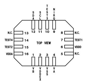
Figure 2-1 Pin Assignments (QFN016)
