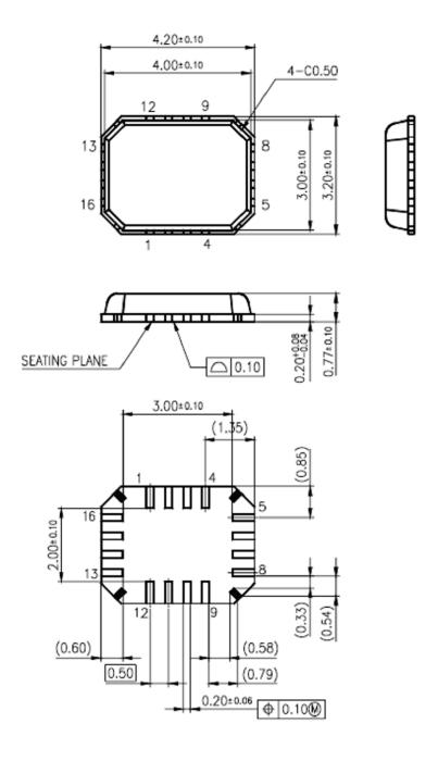
Figure 2-2 Outside drawing (QFN016)
