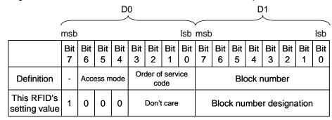
Figure 4-9 Block Element of 2 Bytes
