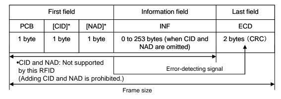
Figure 4-15 ISO/IEC14443-4 Block Format
