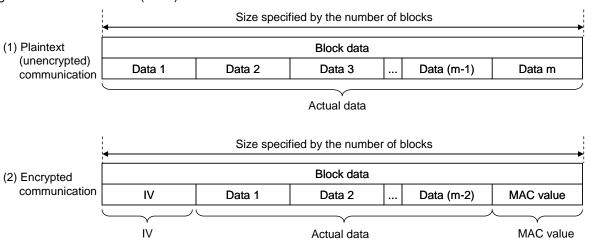
Figure 4-12 Block Data Structure
