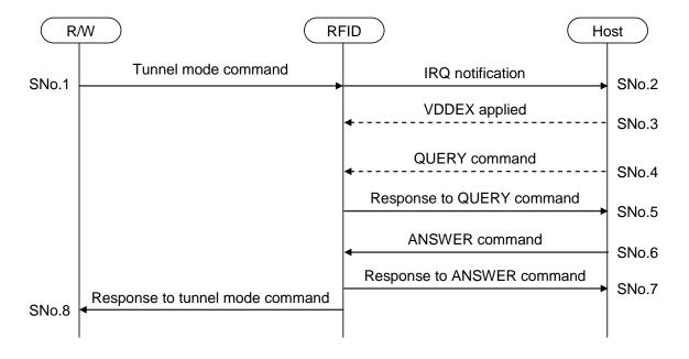
Figure 7-1 Tunnel Mode Sequence
