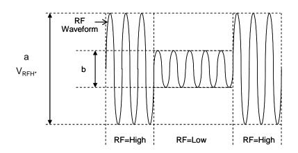
Modulation  $m = \frac{a-b}{a+b}$  The RF a calibra
