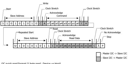
I2C quick read format (1 byte read : Device → Host)
