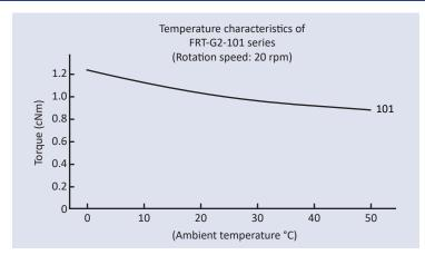
• **Temperature characteristics:** A rotary damper's torque varies according to the ambient temperature. In addition, as shown in the graph above, the torque decreases as the ambient temperature increases, and the torque increases as the ambient temperature decreases. This is because the viscosity of the silicone oil inside the damper varies according to the temperature. When the temperature returns to normal, the torque will return to normal as well.
