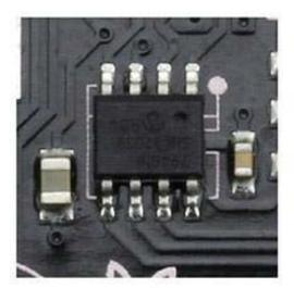
Real Time Clock Keep track of time with the onboard crystal.
