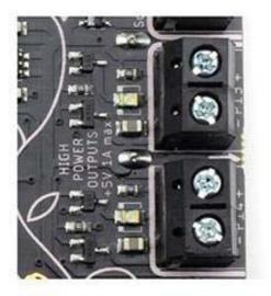
High Power Outputs With these 1A outputs control pumps, fans, heaters and more.
