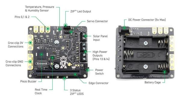
The environmental control board can be coded with the MakeCode editor and Kitronik have produced a set of custom blocks to make the job as simple as possible. There are blocks for reading input and for controlling additional devices such as a pump. This can be added via the add Extensions function in the editor by searching "Kitronik" or from https://github.com/KitronikLtd/pxt-kitronik-smart-greenhouse.
