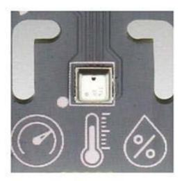
Environmental Sensor Understand the climate by measuring temperature, pressure and humidity.
