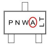
A-Assembly location code: "G"-Qingdao TRS Microelectronics Co. LTD
