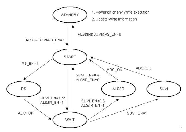
**Note:** When the SUVI sensing enables, all the other sensing will be disable, and their data will remain as previous sensing before SUVI was enable.
