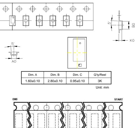
MINIMUM OF 160mm OF EMPTY COMPONENT POCKETS SEALED WITH COVER TAPE.
