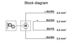
Block diagram of the locking actuator
