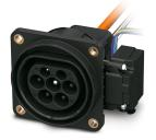
CHARX connect, Vehicle charging inlet, Locking actuator right, For charging electric vehicles (EV) with alternating current (AC), For installation in electric vehicles (EV), AC type 2, IEC 62196-2, length: 2 m, Locking actuator: 24 V, 4-position, M6, Generation 4, A protective cap is supplied as standard for the AC contacts.
