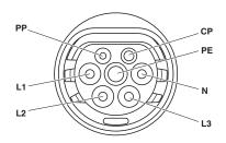
Pin assignment of Vehicle Inlet
