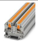
Feed-through terminal block, nom. voltage: 1000 V, nominal current: 41 A, connection method: Push-in connection, Rated cross section: 6 mm<sup>2</sup>, cross section: 0.5 mm<sup>2</sup> - 10 mm<sup>2</sup>, mounting type: NS 35/7,5, NS 35/15, color: gray
