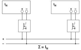
Certain specifications apply in redundancy operation with regard to the configuration of the keepout areas. In redundancy operation, the power supplies are operated with maximum half the nominal power. The keepout areas are therefore reduced.
