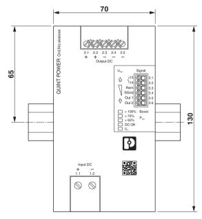
Figure 4 Device dimensions (dimensions in mm)
