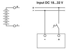
DC applications require upstream installation of a fuse that is permitted for the operating voltage.
