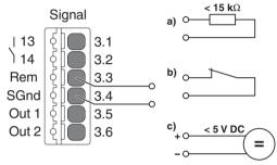
To switch the power supply back on, select one of the following external circuits between signal terminal blocks Rem and SGnd. Power transmission inside the device is activated again. As usual, the energy for supplying the loads is available at the DC output terminal blocks.
