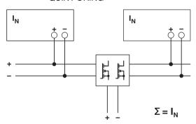
Figure 44 Schematic diagram, redundant operation with QUINT S-ORING
