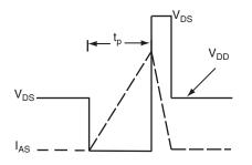
Fig. 12b - Unclamped Inductive Waveforms
