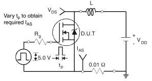
Fig. 12a - Unclamped Inductive Test Circuit
