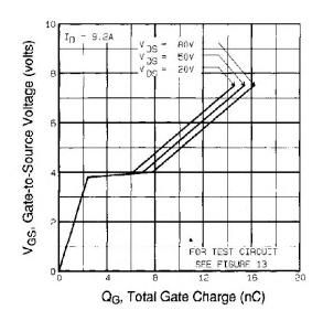
Fig. 6 - Typical Gate Charge vs. Gate-to-Source Voltage
