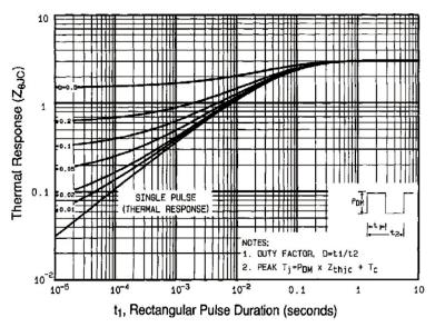
Fig. 11 - Maximum Effective Transient Thermal Impedance, Junction-to-Case
