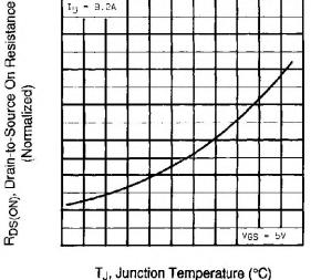
Fig. 4 - Normalized On-Resistance vs. Temperature
