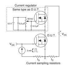
Fig. 13b - Gate Charge Test Circuit
