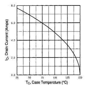
Fig. 9 - Maximum Drain Current vs. Case Temperature
