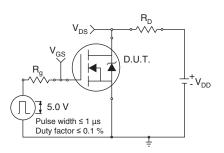
Fig. 10a - Switching Time Test Circuit
