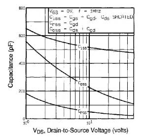
Fig. 5 - Typical Capacitance vs. Drain-to-Source Voltage
