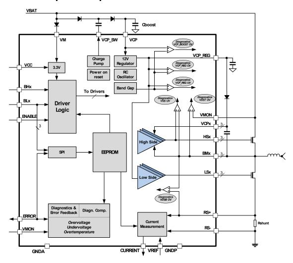
Figure 1.1 Block diagram and principle operation circuit
