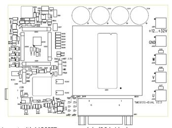
Layout with MOSFET power module (B6-bridge)
