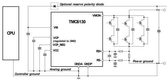
**Figure 1.4 Ground connections**
