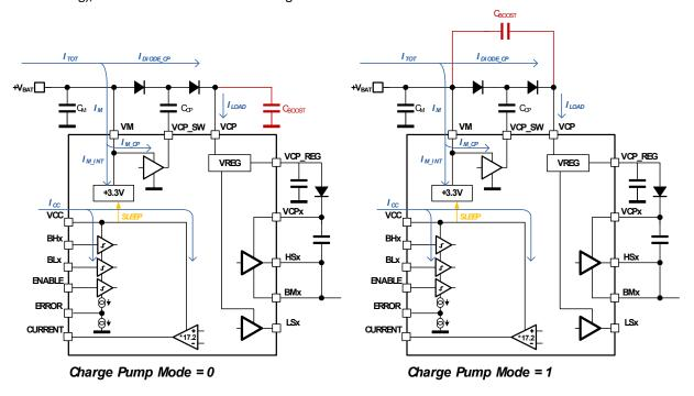
Figure 3.1 Power supply systems: CPMODE = 0 and CPMODE = 1
