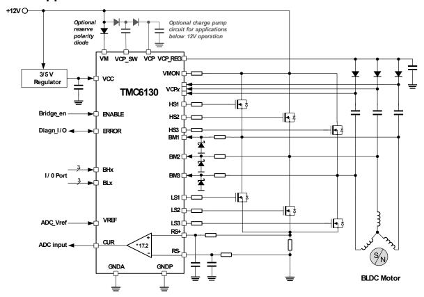
Figure 1.2 Application example for +12V DC
