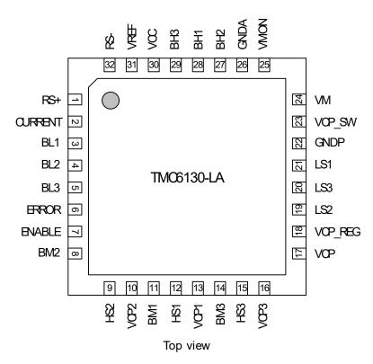
Figure 2.1 TMC6130 pin assignments
