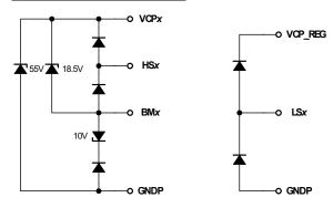
Figure 1.6 Gate driver connections
