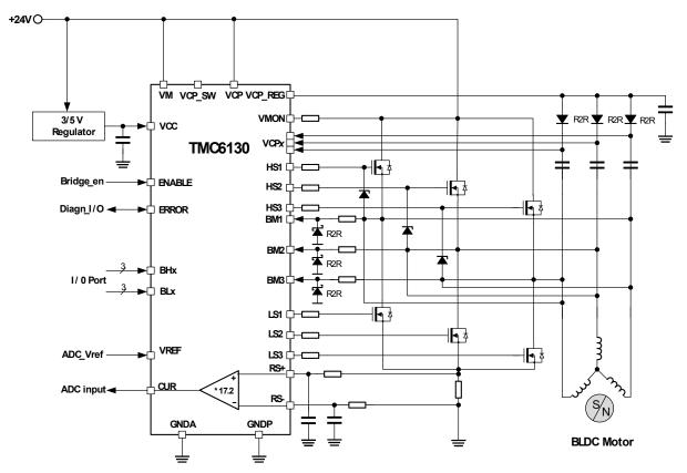
Figure 1.3 Application example for +24V DC
