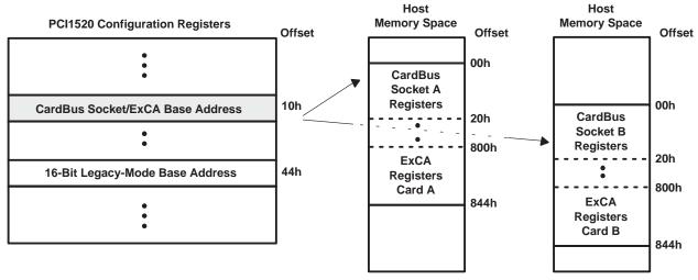
NOTE: The CardBus socket/ExCA base address mode register is separate for functions 0 and 1.
