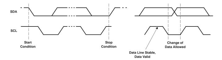
Figure 3-9. Serial-Bus Start/Stop Conditions and Bit Transfers
