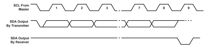
Figure 3-10. Serial-Bus Protocol Acknowledge
