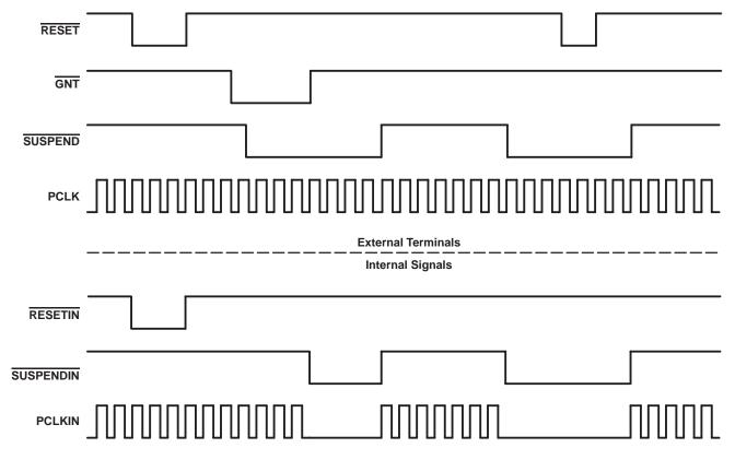
Figure 3-15. Signal Diagram of Suspend Function
