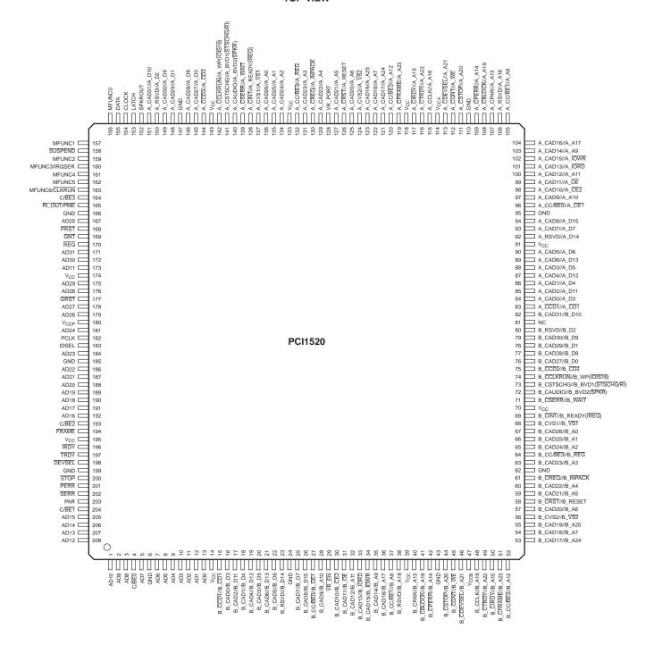
Figure 2–2. PCI1520 PDV-Package Terminal Diagram
