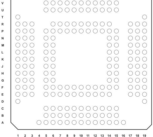
Figure 2-1. PCI1520 GHK-Package Terminal Diagram
