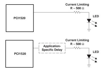
Figure 3-7. Two Sample LED Circuits
