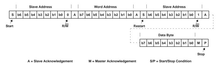
Figure 3-12. Serial-Bus Protocol - Byte Read
