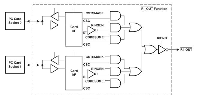
Figure 3–16. RI\_OUT Functional Diagram
