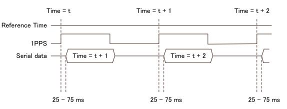
Figure 4.1 Relation between 1PPS, Serial Data and Output Time
