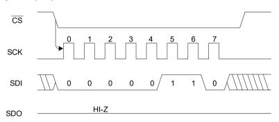
Table 9-1 is a list of actions that will automatically set the Write Enable Latch to zero when successfully executed. If an instruction is not successfully executed, for example if the  $\overline{CS}$  pin is brought high before an integer multiple of 8 bits is clocked, the Write Enable Latch will not be reset.
