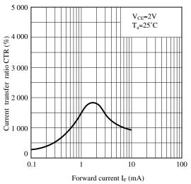
Fig.9 Relative Current Transfer Ratio vs.
