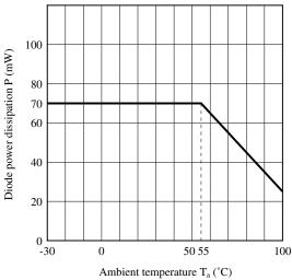
Fig.4 Total Power Dissipation vs. Ambient Temperature
