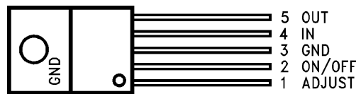
Figure 8. TO-220 5-Lead Power Package Front View
