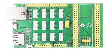
Linklt Smart 7688 Duo is an open development board based on the OpenWrt Linux distribution, MT7688 and ATmega32u4. The board is designed especially to enable the prototyping of Rich Application IoT devices for Smart-Home. If you want to find out more about Linklt Smart 7688 Duo, please click HERE.
