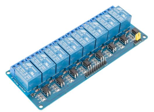
This is a LOW Level 5V 8-channel relay interface board, and each channel needs a 15-20mA driver current. It can be used to control various appliances and equipment with large current. It is equipped with high-current relays that work under AC250V 10A or DC30V 10A. It has a standard interface that can be controlled directly by micro-controller.
