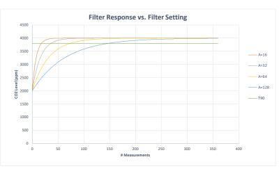
The graph above shows the effect of the filter on response times. Increasing the filter setting increases the measurement output response time.  $T_{90}$  is the time to 90% of reading. The CozIR<sup>®</sup>-LP takes 2 readings per second. The CozIR<sup>®</sup>-LP sensor will also output the raw unfiltered CO<sub>2</sub> measurement data. This data can be post processed using alternative filter algorithms.
