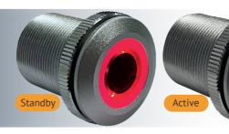
The CTL-SW is a touchless infrared proximity switch, which sits inside a Ø22mm natural anodised aluminium shell. Easily and reliably activated without contact, this proximity switch has a pre-set\* detection range of 4cm. The CTL-SW has onboard LED's showing red when the switch is in standby and green when activated. The momentary action is pre-set\* to 10 seconds.
