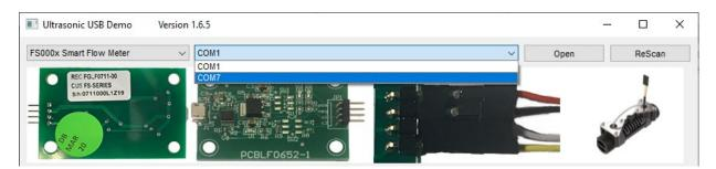
In the case above the hardware was assigned to COM7. Select the new port that was added to Establish communication between the GUI and the pcb.
