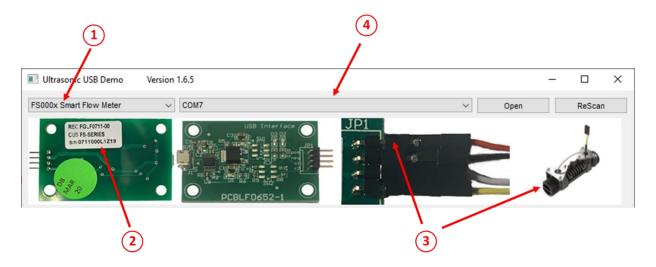
2. Make sure that the correct interface pcb version which supports the FS00xx series is being used. Please note that the same pcb is configured slightly differently for each of the ultrasonic sensors that the GUI supports. For the FS00xx, the white label on the back of the pcb should include the field "FS-SERIES" in the second line as shown as shown below:
