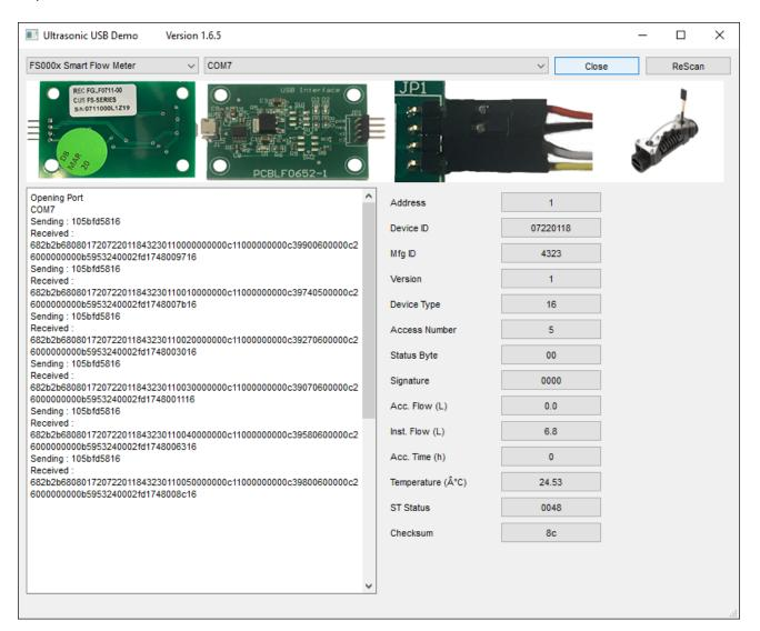
On the left side of the window the actual ASCII data received from the FS Series Flow Meter Module is displayed while on the right side the received data is parsed into the appropriate fields.
