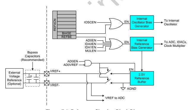
Figure 7.1. Reference Circuitry Block Diagram
