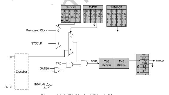
Figure 22.1. T0 Mode 0 Block Diagram
