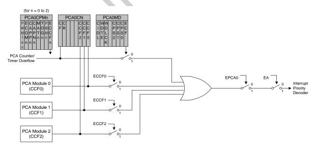
Figure 23.3. PCA Interrupt Block Diagram
