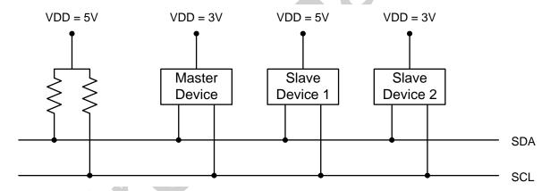
Figure 19.2. Typical SMBus Configuration
