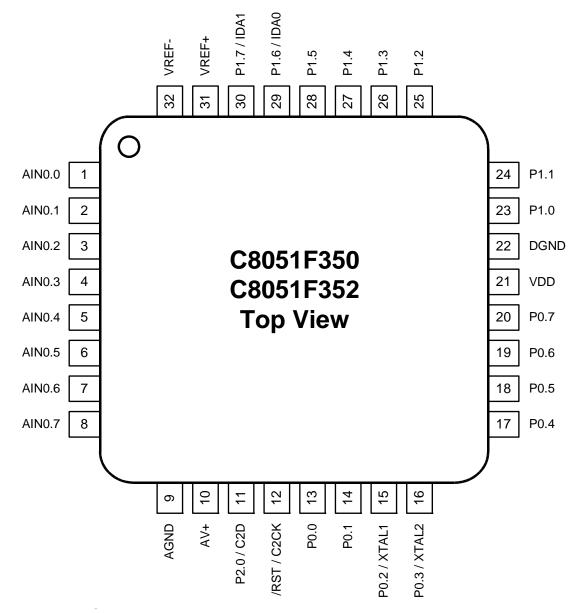
Figure 4.1. LQFP-32 Pinout Diagram (Top View)
