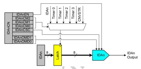
Figure 6.1. IDAC Functional Block Diagram
