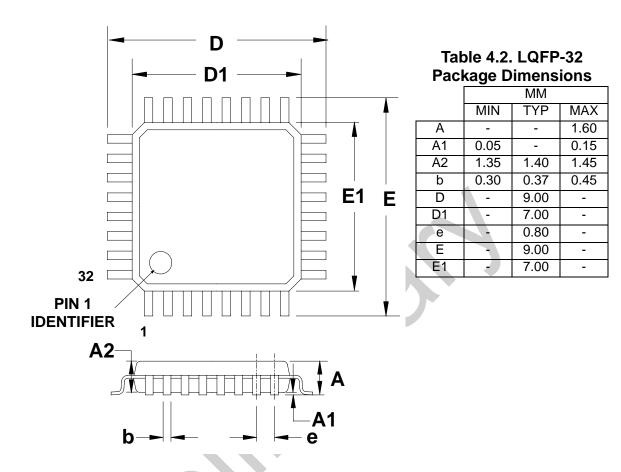
Figure 4.3. LQFP-32 Package Diagram
