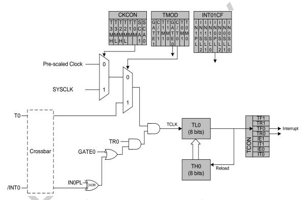
Figure 22.2. T0 Mode 2 Block Diagram
