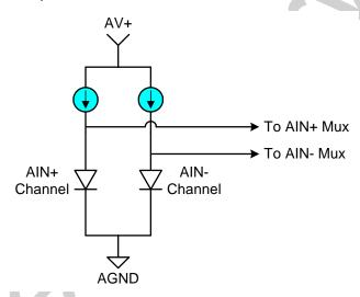
Figure 8.1. Temperature Sensor Block Diagram
