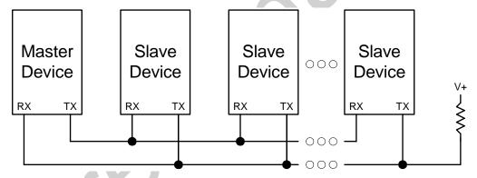
Figure 20.6. UART Multi-Processor Mode Interconnect Diagram
