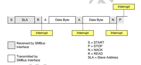
Figure 19.11. Typical Slave Transmitter Sequence
