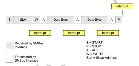
Figure 19.10. Typical Slave Receiver Sequence
