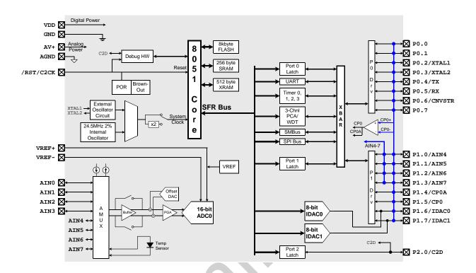
Figure 1.4. C8051F353 Block Diagram
