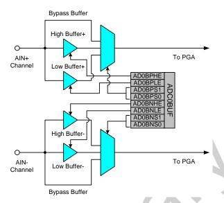
Figure 5.2. ADC0 Buffer Control
