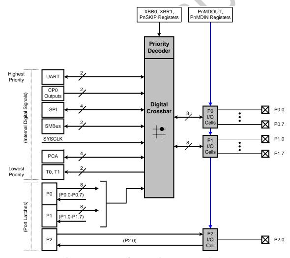
Figure 18.1. Port I/O Functional Block Diagram
