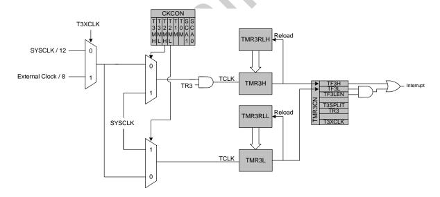
Figure 22.19. Timer 3 8-Bit Mode Block Diagram
