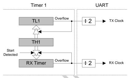
Figure 20.2. UARTO Baud Rate Logic
