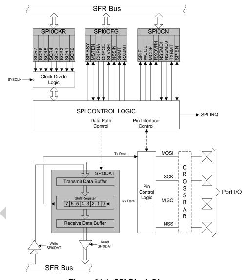
Figure 21.1. SPI Block Diagram
