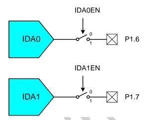
Figure 6.7. IDAC Pin Connections
