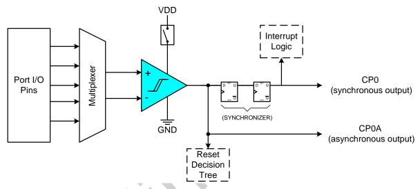
Figure 1.9. Comparator Block Diagram
