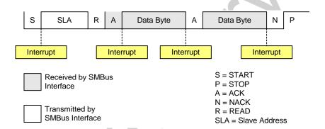
Figure 19.9. Typical Master Receiver Sequence
