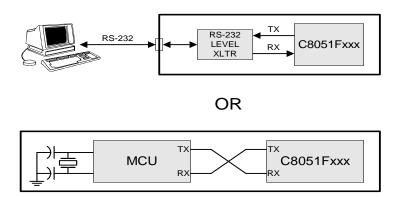
Figure 20.3. UART Interconnect Diagram
