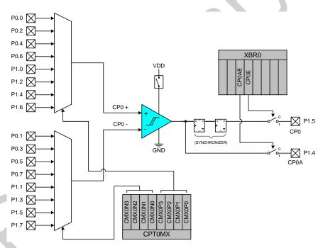
Figure 9.5. Comparator Pin Connections
