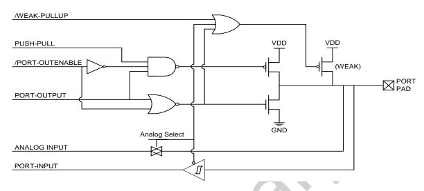
Figure 18.2. Port I/O Cell Block Diagram
