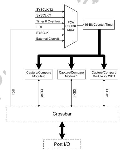
Figure 23.1. PCA Block Diagram
