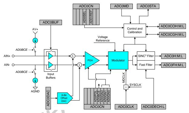
Figure 5.1. ADC0 Block Diagram
