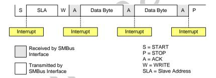
Figure 19.8. Typical Master Transmitter Sequence
