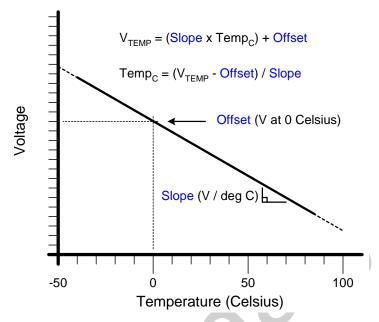
**Figure 8.2. Single Channel Transfer Function**
