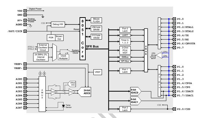
Figure 1.1. C8051F350 Block Diagram
