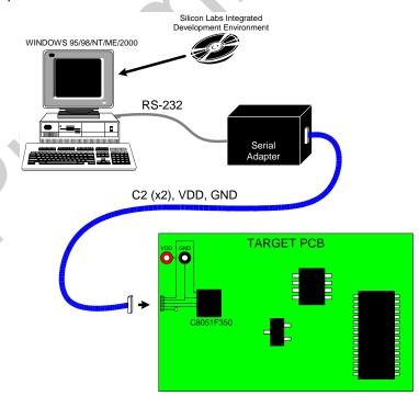
Figure 1.5. Development/In-System Debug Diagram
