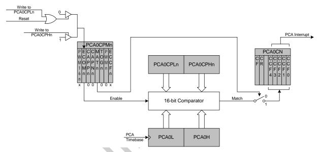
Figure 23.5. PCA Software Timer Mode Diagram
