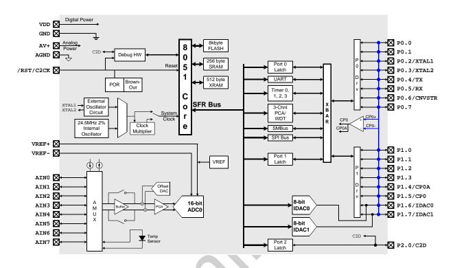
Figure 1.3. C8051F352 Block Diagram
