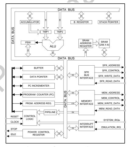
Figure 10.1. CIP-51 Block Diagram
