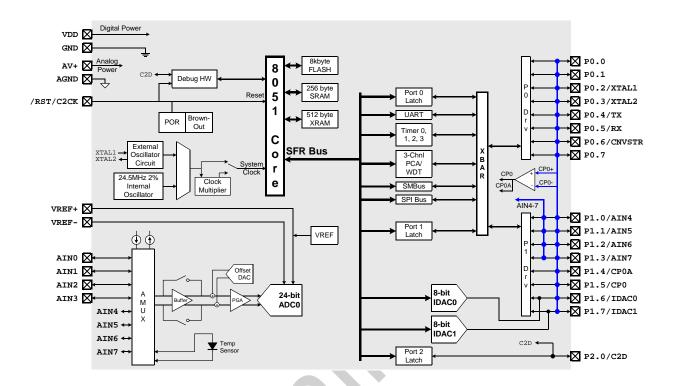
Figure 1.2. C8051F351 Block Diagram
