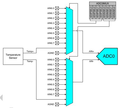
Figure 5.26. ADC0 Multiplexer Connections
