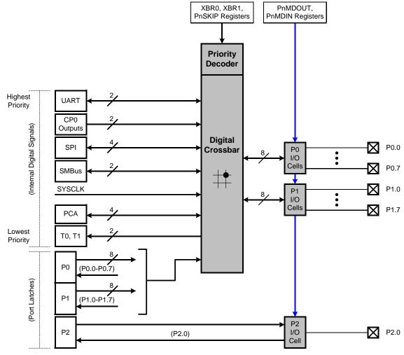
Figure 1.10. Port I/O Functional Block Diagram
