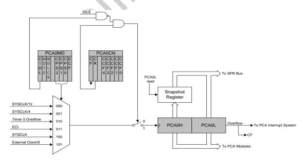
Figure 23.2. PCA Counter/Timer Block Diagram
