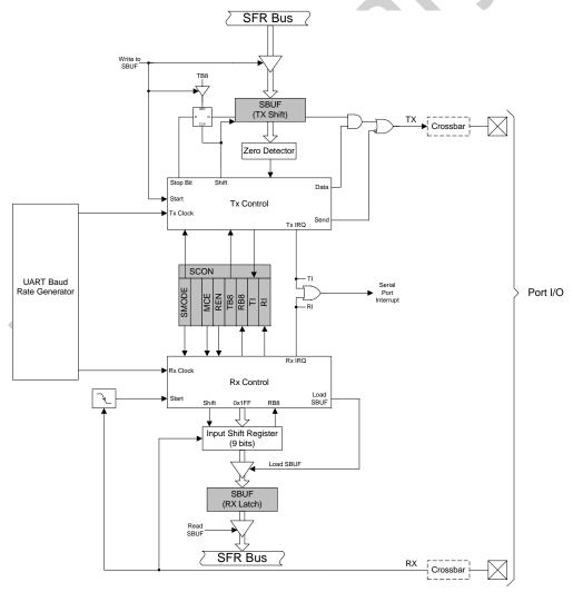
Figure 20.1. UARTO Block Diagram
