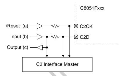
Figure 24.6. Typical C2 Pin Sharing
