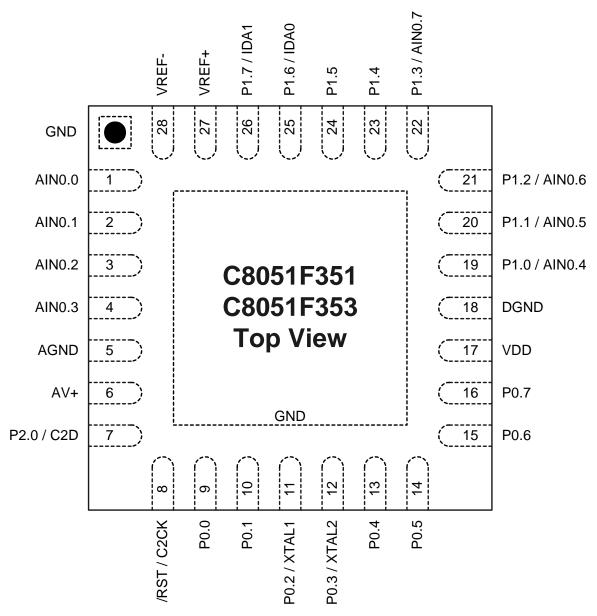
Figure 4.2. MLP-28 Pinout Diagram (Top View)
