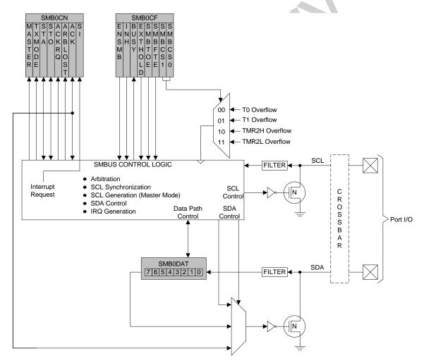
Figure 19.1. SMBus Block Diagram
