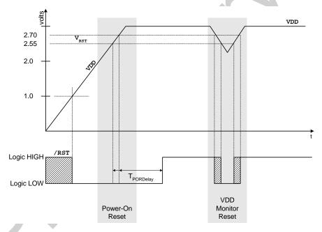
Figure 14.2. Power-On and V<sub>DD</sub> Monitor Reset Timing
