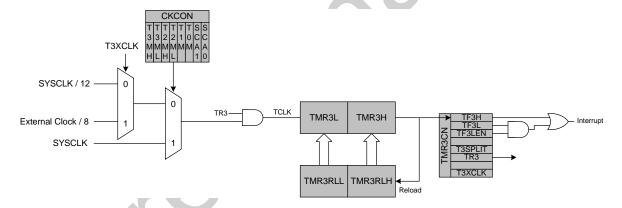
Figure 22.18. Timer 3 16-Bit Mode Block Diagram
