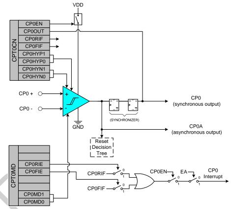
Figure 9.1. Comparator Functional Block Diagram
