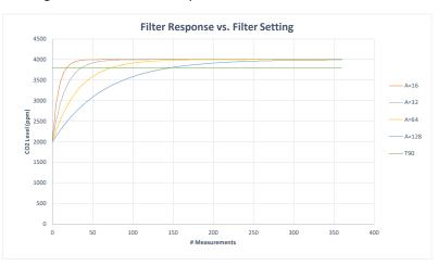
The graph above shows the effect of the filter on response times. Increasing the filter setting increases the measurement output response time.  $T_{90}$  is the time to 90% of reading. The CozIR<sup>®</sup>-A takes 2 readings per second.
