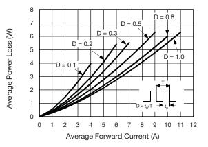
Fig. 2 - Forward Power Loss Characteristics Per Diode
