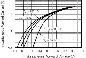
Fig. 3 - Typical Instantaneous Forward Characteristics Per Diode
