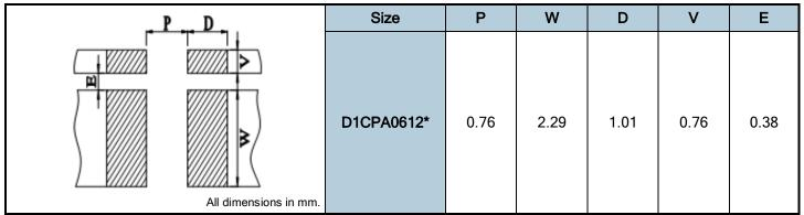
Note: PCB material is FR4. Board thickness is 1.10mm. 1 oz. copper used on current sense resistor placement layer.
